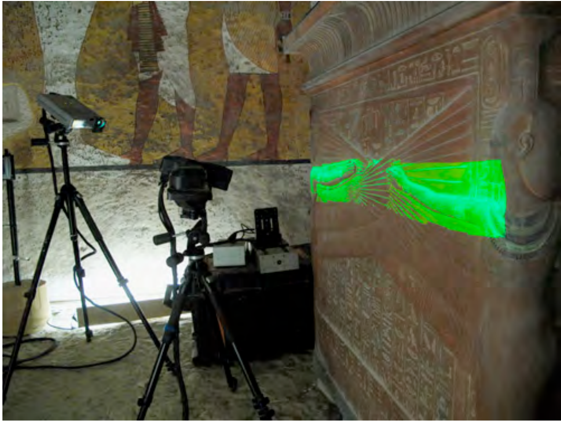
Nub 3D structured light scanner recording the west side of the sarcophagus.
